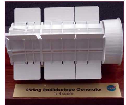
A quarter-size model of a Stirling Radioisotope Generator - designed to produce 140 watts of electric power in the cold, deep reaches of outer space for over 17 years of unattended and no maintenance operation - a gift from Robert Cataldo of the National Aeronautics and Space Administration.
